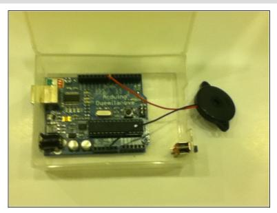
To assemble this project, simply plug the speaker into the Arduino, with the positive pin going to pin 8 and the negative to ground. Also, plug in the Arduino to your computer.
